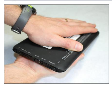
After you have removed the screws from the bottom of the tablet, you can now slide the cover off. To do this, place your hand on the panel and firmly slide the panel in the direction that the arrow indicates.
