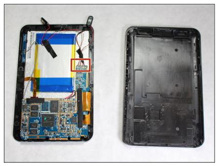
• Next, find the wires that connect the speakers to the motherboard. (Follow the red marker indicated in the image.) To remove these, you will use the soldering iron.
