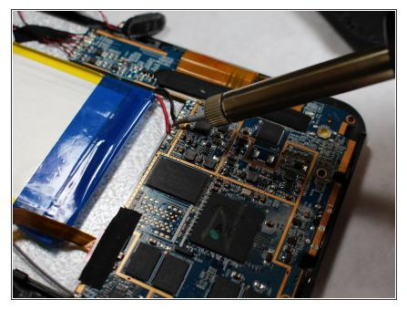
• <u>Desolder</u> the two wires connecting the battery to the mother board.
