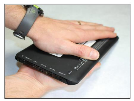
• Firmly slide the cover in the direction indicated by the arrow, away from the ports, with your hand to remove the back cover.
