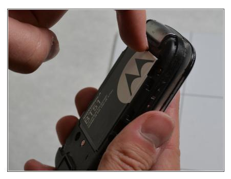
• Use the tab located at the top of the battery to release the battery.
