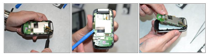
• Remove the flex cable with a pair of tweezers.
