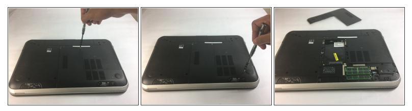
• Take your screwdriver and loosen the three 4mm screws to remove the cover.
