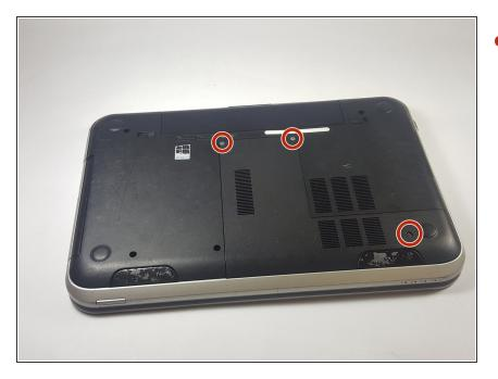
Locate RAM compartment on device and corresponding screws.
