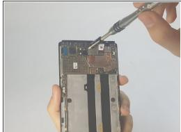
• Remove the 3.15mm Phillips Head #000 screws from motherboard.
