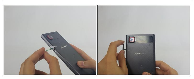
Remove the SIM card tray by pushing a pin into the hole on the side of the phone.
