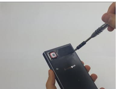
Remove the 4.9 mm torx head screws located on the camera plate on the back of the phone
