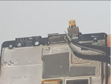
• Gently lift the speaker out of its housing by inserting the tweezers under the speaker.
