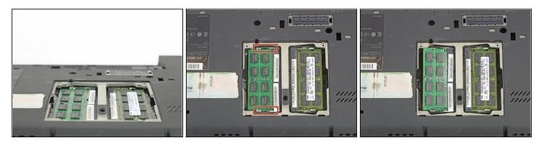
• Push the marked claws to the side, to make the RAM accessible.
