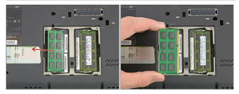
• To remove the RAM, you need to pull the RAM into the shown direction out of its connector.
