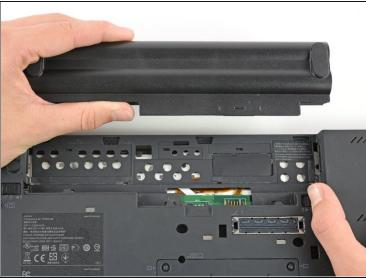
Now push and hold the right switch to the right while using the other hand to gently slide the battery upwards out of the laptop.
