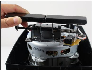
Lift out the button assembly by pulling up.
