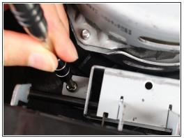
Remove the two 13.0mm screws that are holding down the button assembly using the Phillips #2 screwdriver.
