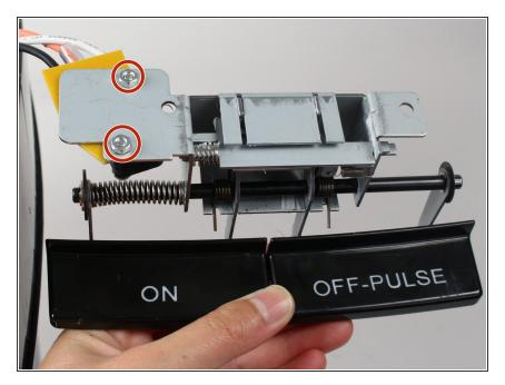
Remove the two 5.5mm nuts with a 5.5mm nut driver.
