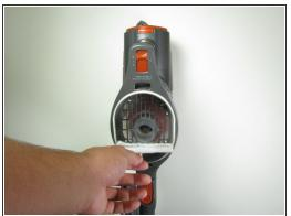
Remove the the outer and inner filters inside the vacuum by pulling them out.
