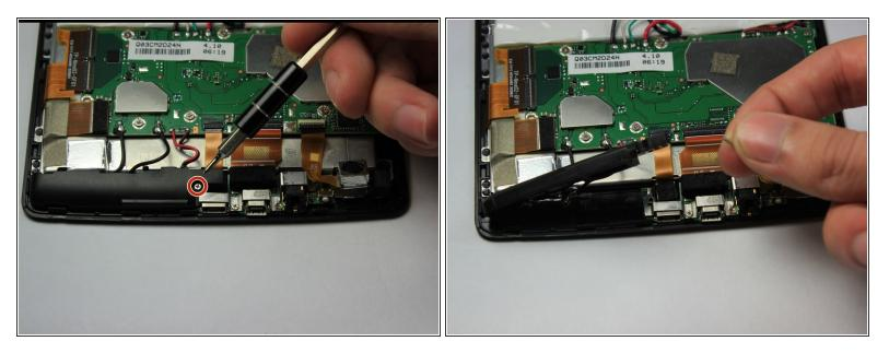
• Use the PH #000 phillips screw bit to remove one 5.0 mm screw.
