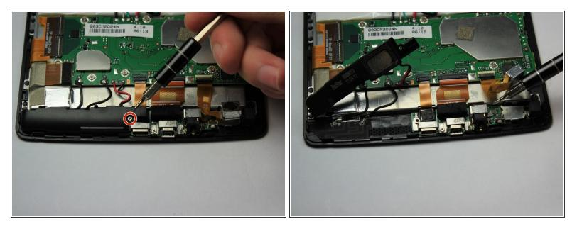
Use the PH #000 screw bit to remove the 5.0 mm screw holding down the top speaker to expose the front-facing camera.
