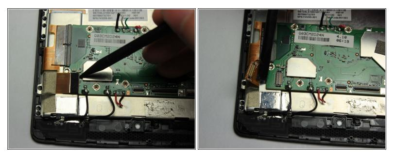
Disconnect the press-fit connector from the mother board using the nylon spudger. Gently pry the connector up; it will pop out of place easily, so if its not coming out don't force it.
