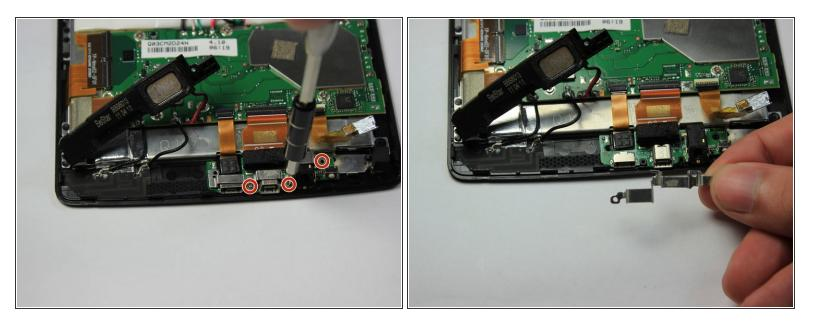
Use the PH #000 phillips head screw driver to remove three 3.0mm screws. Remove the silver bracket.
