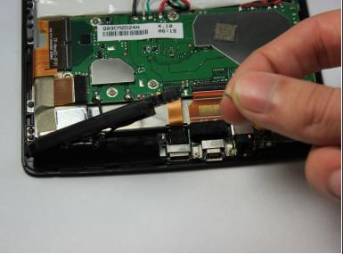
Use the PH #000 phillips screw bit to remove one 5.0 mm screw.
