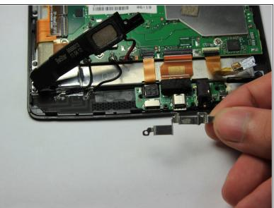
Use the PH #000 phillips head screw driver to remove three 3.0mm screws. Remove the silver bracket.
