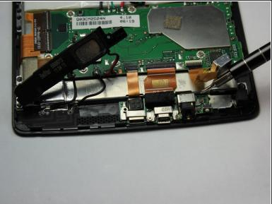
• Use the PH #000 screw bit to remove the 5.0 mm screw holding down the top speaker to expose the front-facing camera.
