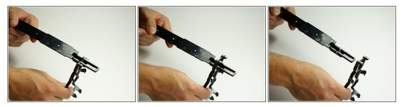
• Lift the lever arm from the slot it is in and slide off of the end of the plastic piece that was holding it to the boat.
