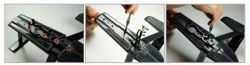
• Remove the four remaining 1cm screws with the T8 screw driver.
