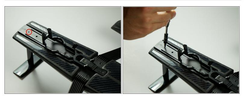
• Remove the far left 1cm screw using a T8 screwdriver.
