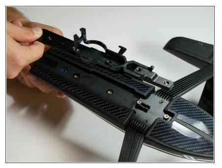
• Lift up on the plastic piece that is securing the lever arm.
