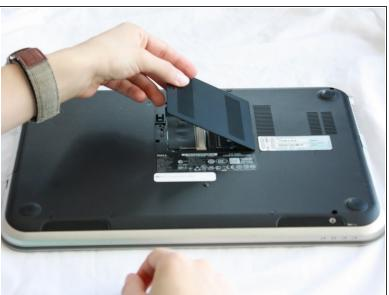
Lightly lift the RAM cover up and at an angle, away from the computer.
