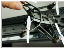
• Use your pointer finger on one tab, your middle finger on the other, and your thumb on the bottom to pry the tabs away and lift the drone out of the holder.
