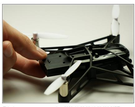
Pull the battery fully out using your fingers.
