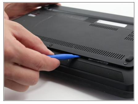
Using a small plastic opening tool, pry off the back casing starting at a point closest to you and working around the perimeter of the case.
