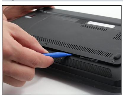
Using a small plastic opening tool, pry off the back casing starting at a point closest to you and working around the perimeter of the case.
