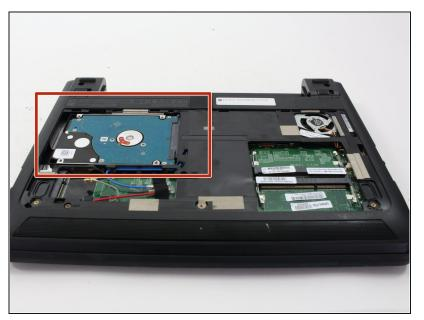
After removing the back panel, locate the hard drive located to the far left. It is distinguishable from other parts based on it's rectangular shape.
