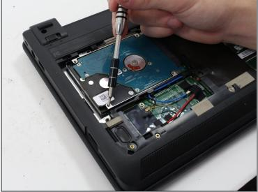
• Remove the four 3.5 mm Phillips #0 screws attached on the four corners of the hard drive.
