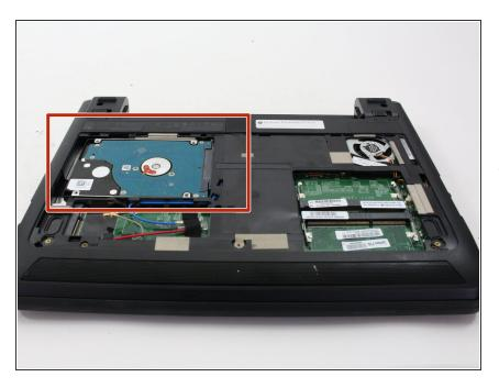
After removing the back panel, locate the hard drive located to the far left. It is distinguishable from
