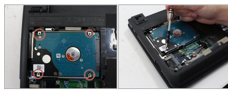
Remove the four 3.5 mm Phillips #0 screws attached on the four corners of the hard drive.
