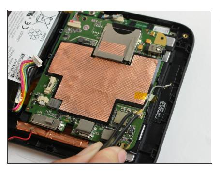
Use tweezers to disconnect the ground wire from motherboard terminal.
