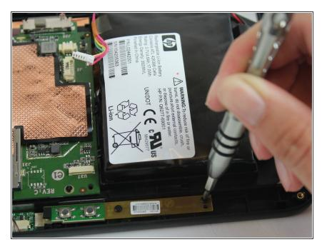
• Remove the two 6 mm screws using a Philips #0 screwdriver.
