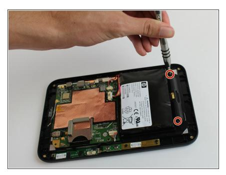
Remove the two 6mm screws using a Phillips #0 screwdriver.
