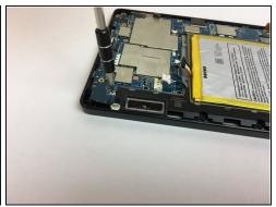
• Remove the nine silver screws located around the motherboard with the T5 Torx screwdriver.
