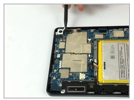
Use a nylon spudger to unclip the connection from the motherboard.
