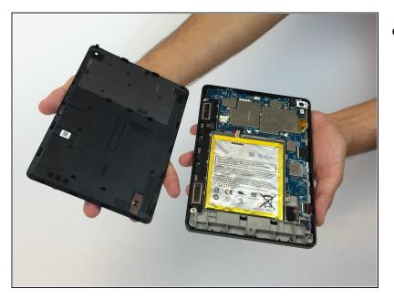
• Once all clips have been released, remove the back case to reveal the inside of the device.
