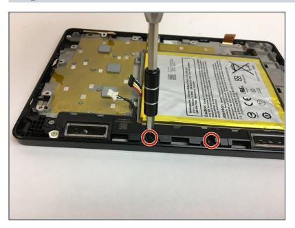
• Remove the two black screws using the T5 Torx screwdriver.
