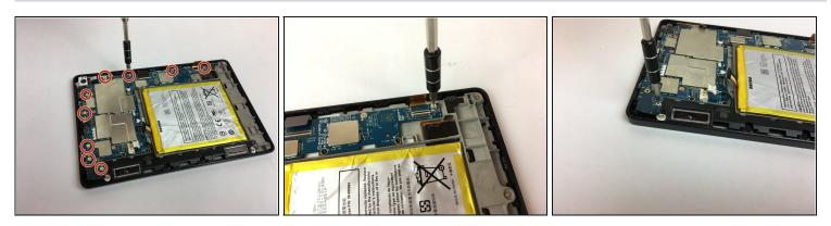
• Remove the nine silver screws located around the motherboard with the T5 Torx screwdriver.
