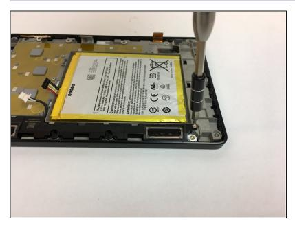
• Remove the single silver screw with the T5 Torx screwdriver.
