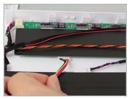
Disconnect the wires from the power regulator by pulling the white connector straight out.
