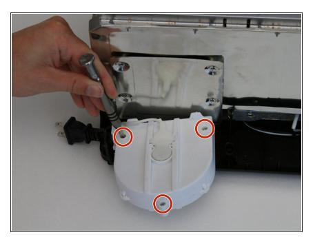
Use the PH#1 bit to remove the three 8mm screws located on the back side of the casing.
