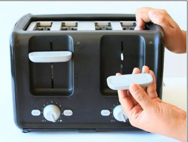
Forcefully pull the slot lever away from the toaster by keeping parallel to the table.
