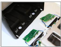
Use a J1 screw bit to unscrew eight 8mm screws from the motherboard.
