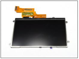
Separate the display from the digitizer. The display is now fully removed from the device.
