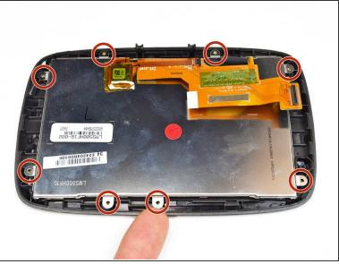
Unscrew the eight 2.5mm screws along the perimeter of the display using the Phillips #000 screwdriver.
