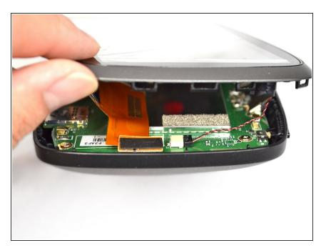
With the screen casing unlatched, locate the right side where the two connectors are.
