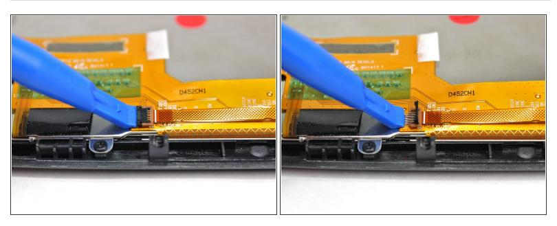
Lift up the small black tab on the orange connector using a plastic opening tool. This releases the strip connecting the display to the digitizer.
