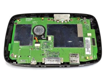
Separate the screen casing from the motherboard casing.
