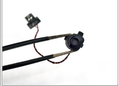
Remove the microphone on the left side of the screen casing using tweezers.
