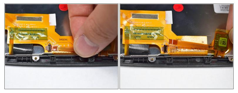
Slide the connector strip out from the tab.
