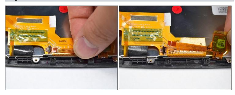
• Slide the connector strip out from the tab.
