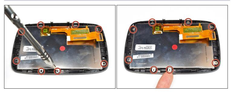
• Unscrew the eight 2.5mm screws along the perimeter of the display using the Phillips #000 screwdriver.
