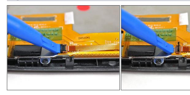
• Lift up the small black tab on the orange connector using a plastic opening tool. This releases the strip connecting the display to the digitizer.
