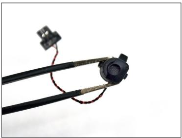
• Remove the microphone on the left side of the screen casing using <u>tweezers</u>.
