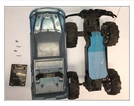
Using a big phillips screwdriver unscrew the housing that holds the wheels
