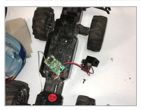
Use a small phillips screw driver to unscrew the circuit board
