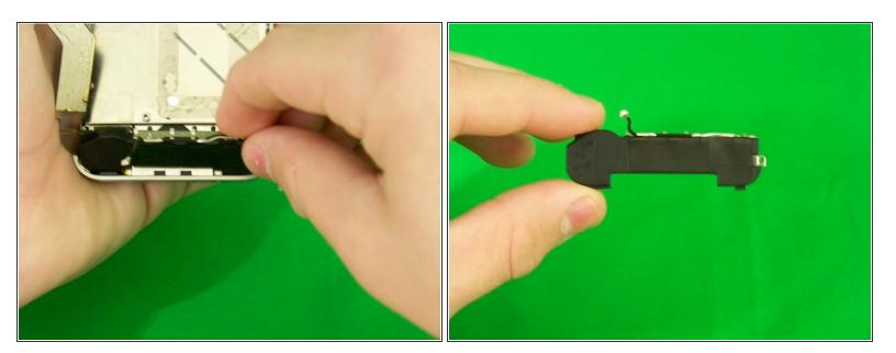
Using the plastic opening tools or your fingers pull up on the speaker enclosure.
