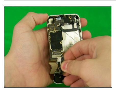
Using your fingers or a plastic opening tool carefully pull out the logic board.
