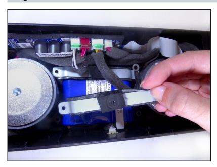
Remove the two brackets that hold down the battery using your hands.
