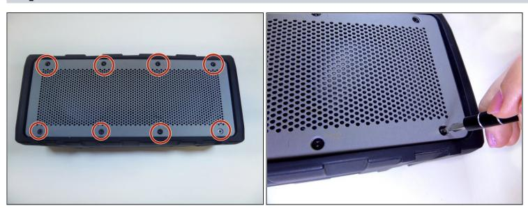
• Placing the device with the back panel facing up, remove the eight 5mm hexagon 2.0 screws from the back panel.
