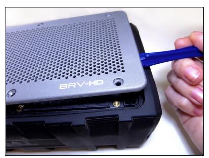
Lift the front panel off of the speaker using a plastic opening tool.
