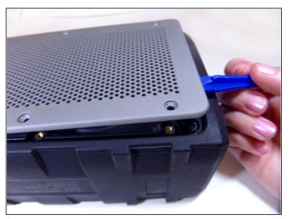
Lift the back panel off of the device with a plastic opening tool.
