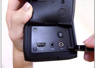
• Turning the device on its side, unscrew the four 15mm hexagon 2.0 screws on the charging port panel.
