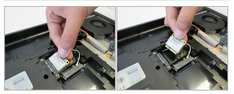
Remove the wireless module from the laptop.
