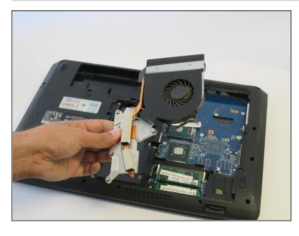
• Install the modified or new cooling fan.
