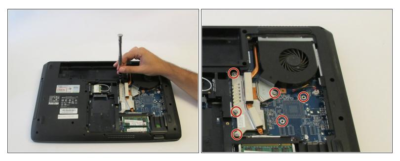
Use the Phillips #1 screwdriver to unscrew the four Phillips #1 screws that connect the cooling fan from the panel.
