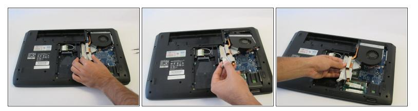
• Carefully remove the cooling fan from the motherboard.
