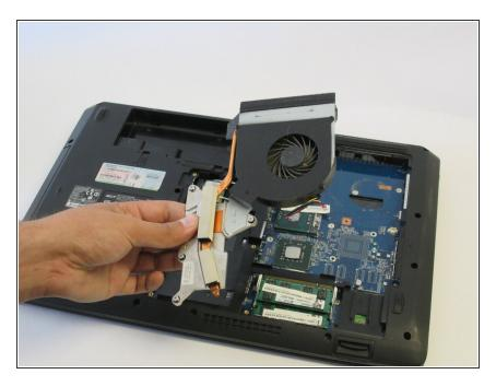
Install the modified or new cooling fan.
