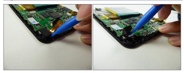
• Use a plastic opening tool to remove the camera.
