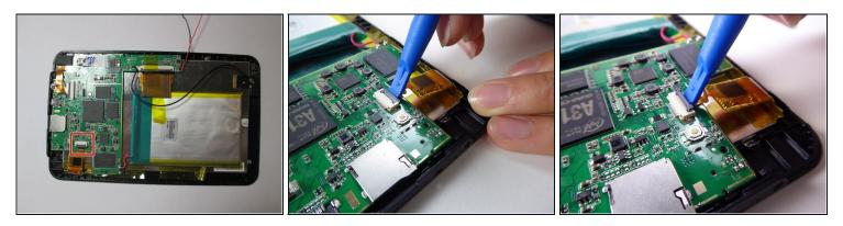
• Use a plastic opening tool to lift the black tab.
