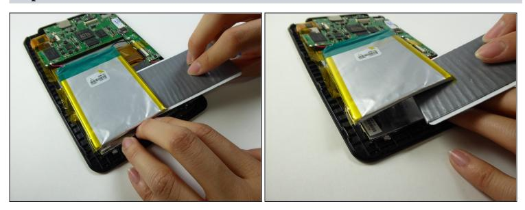
• Wedge a <u>plastic card</u> underneath the battery to remove it.
