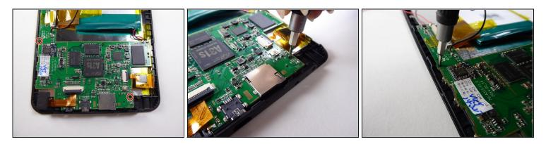
• Use a Phillips #000 screwdriver to remove the two 3.6mm screws.
