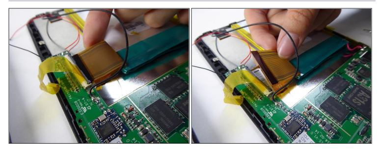
• Carefully lift and remove the ribbon cable from the black tab.
