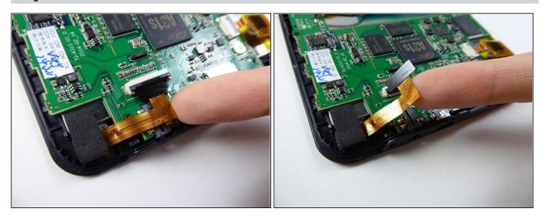
• Carefully lift and remove the ribbon cable from the black tab.
