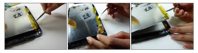
Wedge a metal spudger underneath the LCD screen to remove it.
