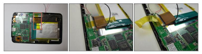
• Lift the tape holding down the battery.
