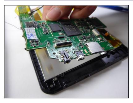
Safely remove the battery and motherboard from the tablet.
