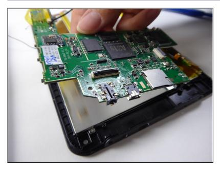
• Lift to remove the battery and motherboard from the tablet.
