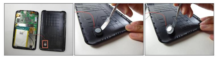
• Wedge a curved metal spudger to remove the speaker.
