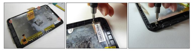
• Use a Phillips #000 screwdriver to remove the three 2.5mm screws.
