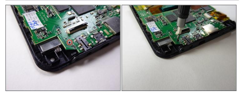
• Use a Phillips #000 screwdriver to remove the 3.6mm screw.
