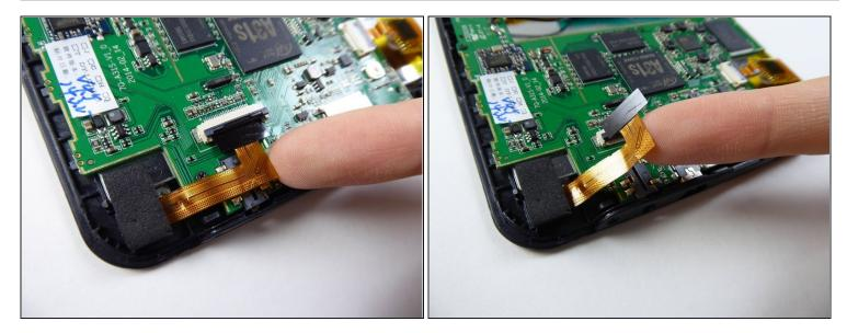
• Carefully remove the ribbon cable from the black tab.
