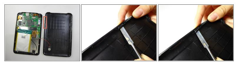
Using a metal spudger and/or your fingers, press the power button in and lift the outside tab.
