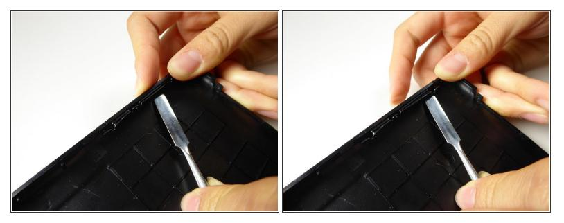
Using a metal spudger and/or your fingers, press the volume button in and lift the outside tab.
