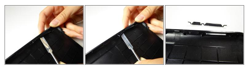
Using the metal spudger, dislodge and lift the power and volume buttons
