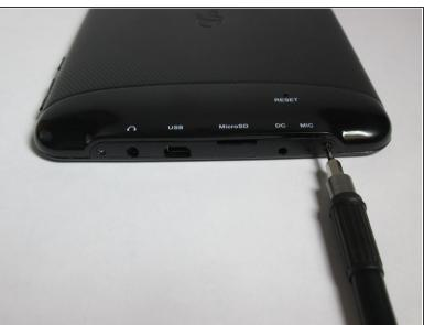
At the bottom of the tablet, remove the two 3.6mm screws with a Phillips #000 screwdriver.
