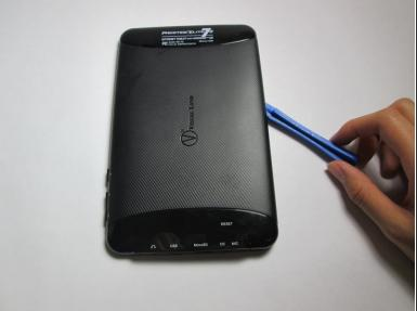
Wedge a plastic opening tool into the edges of the tablet to pry it open.
