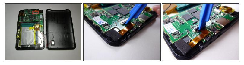
• Use a plastic opening tool to lift the black tab holding down the ribbon cable.
