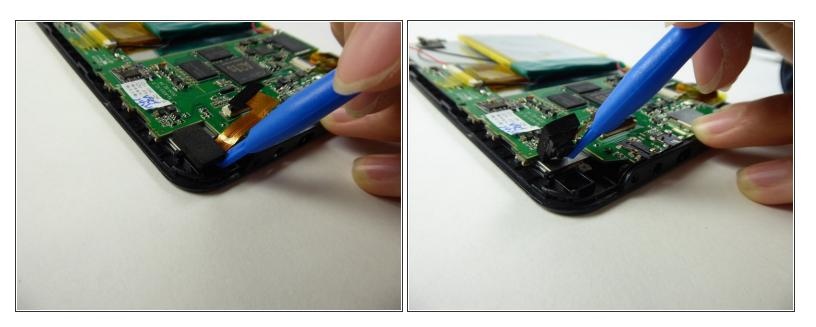
Use a plastic opening tool to pull out the camera with the foam backing.
