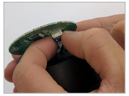
• Pull black piece on top of socket away from board to loosen, then detach the cable.
