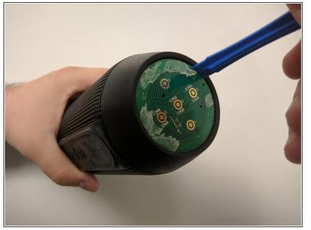
Use your plastic opening tool to pry the button board loose by lifting the edges.
