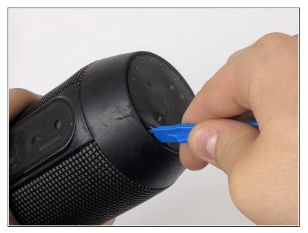
• Use a plastic opening tool to pry around the edges of the circular rubber panel.
