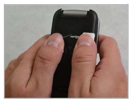
• Slide the tab off the back of the device.
