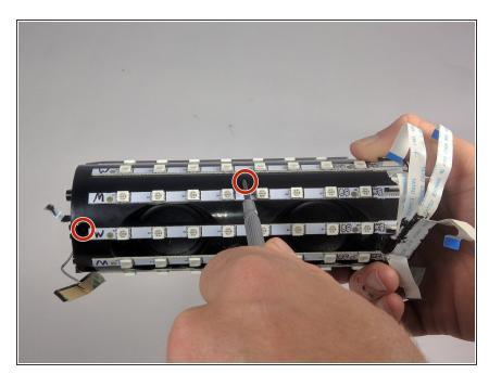
Remove two black 9mm PH0 screws from outside of inner casing on each side.
