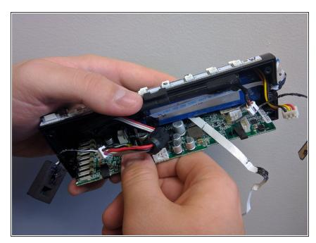
Once all of the cables are removed, grip the motherboard and slide it out.
