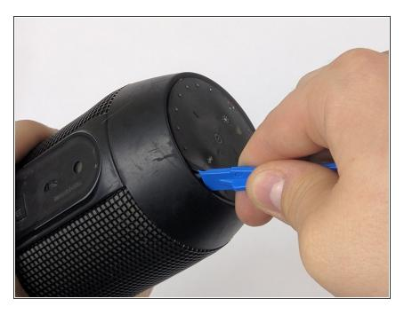
Use a plastic opening tool to pry around the edges of the circular rubber panel.
