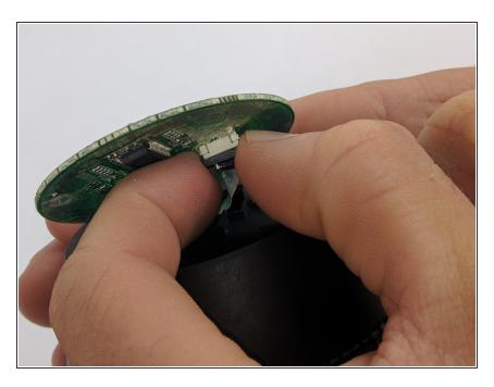
Pull black piece on top of socket away from board to loosen, then detach the cable.
