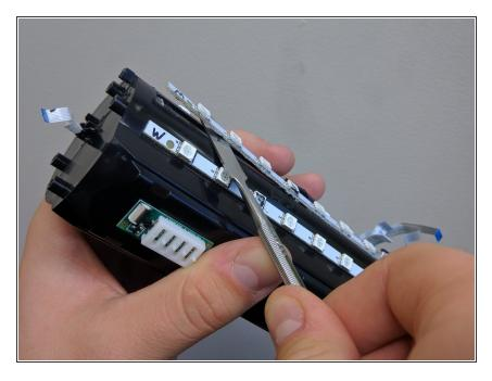
Pry off LED light panel using a metal spudger. To reassemble your device, follow these instructions in reverse order.
