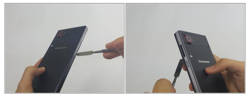
Push the Spudger along the gap between the phone and the backplate to separate them.
