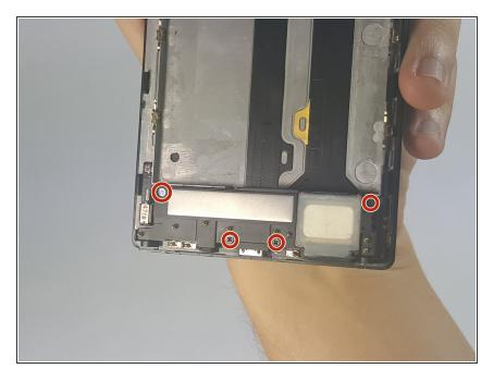
Remove the 3.6 mm Phillips head screws from the charging assembly
