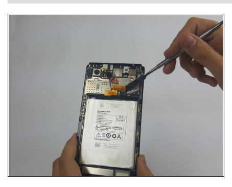
Disconnect the orange battery ribbon cable by gently lifting with a spudger.
