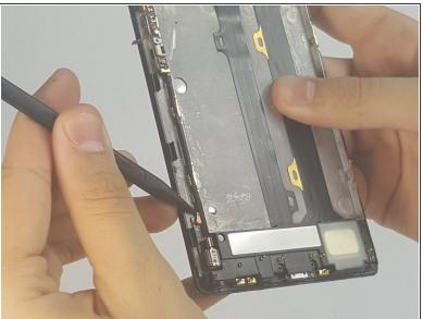
Remove the antenna connected to the bottom piece of the screen plate
