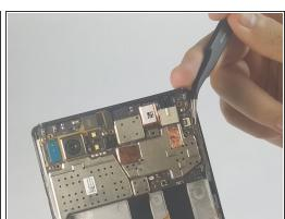
Disconnect the two ribbon cables by gently lifting on the black hinges and pulling away with tweezers
