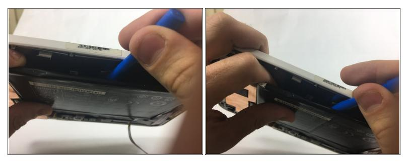
• Carefully break the bond between the inner tape and the battery using the plastic opening tool. The tape can be found in the middle and either side of the battery.
