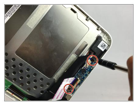
Unscrew the 3mm phillips head screws connecting speaker and home button circuit board from main frame using the HHO screwdriver.
