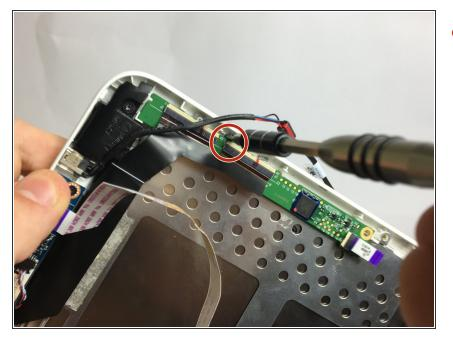
Unscrew the 3mm phillips head screws from beneath the screen circuit board using the same HHO screwdriver.
