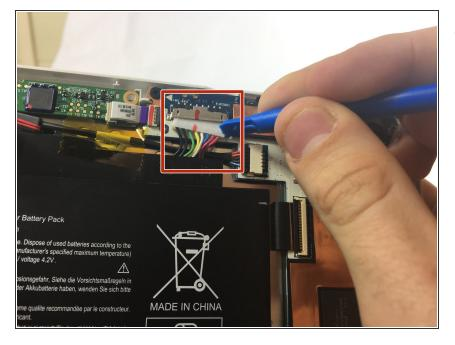
Use the plastic opening tool to carefully slide the power cord from its slot by pushing it out from both sides, then remove the cord from its port with your hand.
