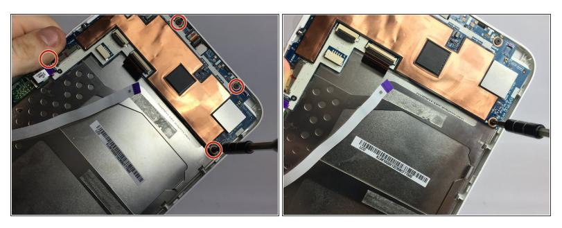
• Unscrew the 3mm phillips head screws along the motherboard using a HH0 screwdriver.
