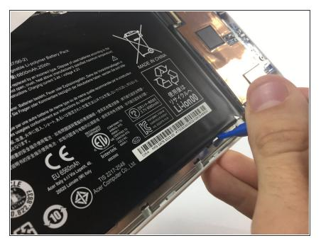
Use the plastic opening tool to gently wedge out and lift the battery pack from the device.
