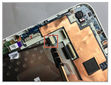
• Disconnect the speaker cord from the motherboard by carefully prying it out with a plastic opening tool.
