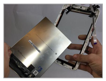
• Remove the screen from the front casing.
