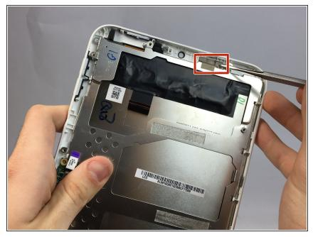
• Loosen metal tape from the front panel using a spudger.
