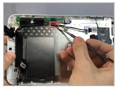
Loosen speaker cord from main back frame by breaking the tape seal using a spudger.
