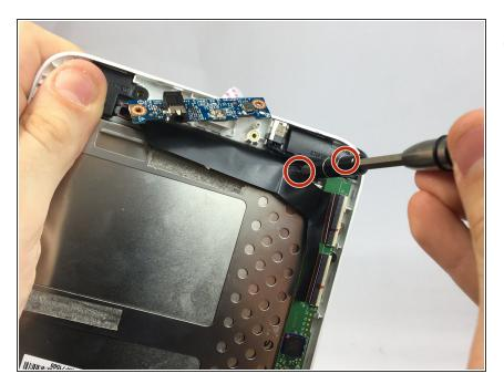
Unscrew left speaker from frame by moving the ribbon cord out of the way to access the 3mm phillips head screws.
