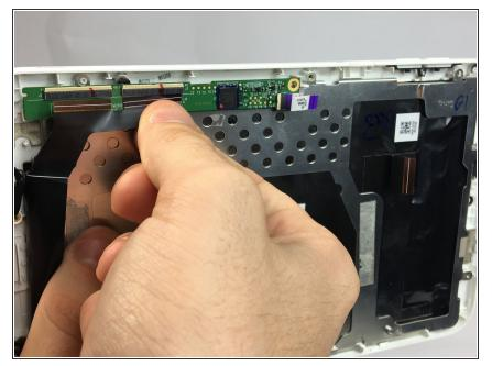
• Pull ribbon cord from designated slots on screen circuit board.
