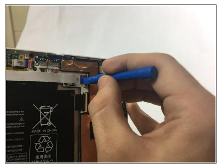
• Pull the ribbon cord by pushing the clamp on the port toward you with the plastic opening tool.
