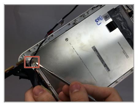
• detach metal tape from the back of the screen using a spudger.
