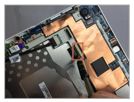
Loosen the retaining flap using a plastic opening tool, and then pull the ribbon cord from its slot.
