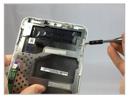
• Loosen the main back metal frame from the front casing using a plastic opening tool.
