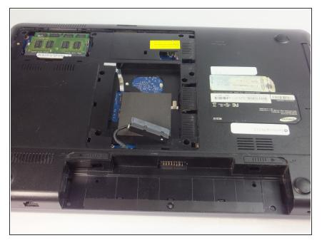
• Take out the HDD and leave the connector in the laptop
