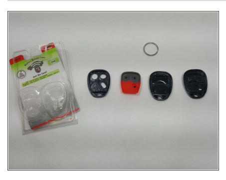
After Opening the new Key Fob package, select the correct housing as more than one model is included.
