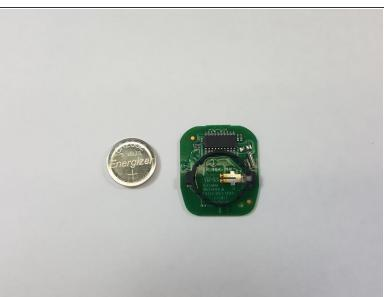
If necessary, remove the battery from the electrical board and replace it.
