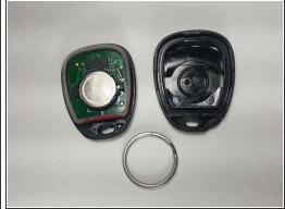
Once you have removed the key ring, use it to open the housing by wedging it into the groove, as pictured.
