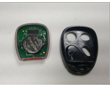
Remove the electrical board and rubber key pad from the old housing.
