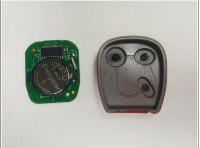
Remove the electrical board from the rubber key pad.
