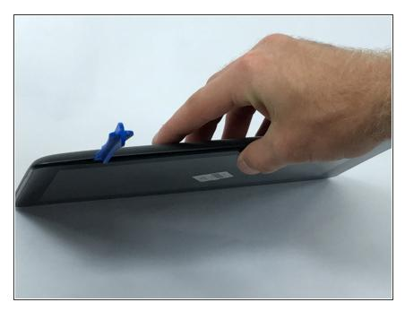
Slide the plastic opener around the tablet. There will be spots of resistance. These should gently pop open as the tool slides through the seam.
