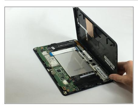
After all of the clips have been opened, the back panel should be free to remove by hand
