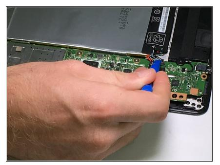
Using the blue plastic opening tool unplug the battery plug by gently pushing the plug out parallel to the motherboard.
