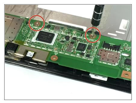
Using the PH00 screwdriver, remove the 2 silver M2x2mm screws along the top of the motherboard.
