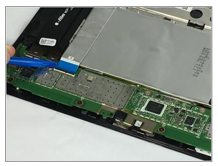
Use the blue plastic opening tool to lift open the black latch connecting the blue ribbon cable to the motherboard.
