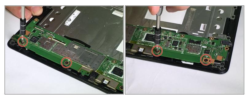
Using the PH00 screwdriver, remove the 4 black M2x4mm screws along the bottom of the motherboard.
