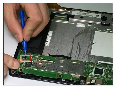
Unplug the speaker cable by gently pushing it parallel to the motherboard with the flat side of the blue plastic opening tool.
