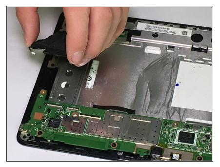
• Lift the speaker up by the end opposing the steel latch and slide it out from under the steel latch. The speaker has now been removed.
