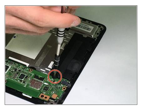
• Unscrew the M2x4mm screw with the PH00 screwdriver attachment.
