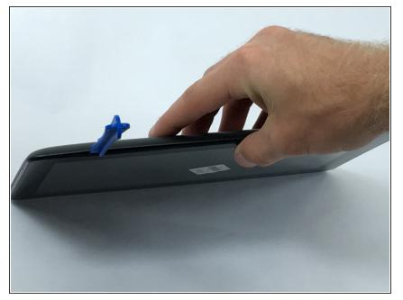
Slide the plastic opener around the tablet. There will be spots of resistance. These should gently pop open as the tool slides through the seam.
