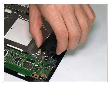
• Lift the speaker up by the end opposing the steel latch and slide it out from under the steel latch. The speaker has now been removed.
