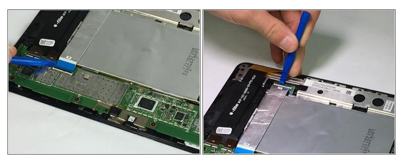
Unplug the blue ribbon cable which runs across the top of the battery near the left-hand speaker. It
